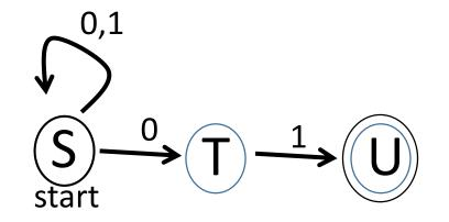
In general, an NFA is a quintuple (Q,  $\Sigma$ ,  $\delta$ , s, F) where Q,  $\Sigma$ , s, and F have the same meanings as in a DFA, and for each state t and letter a in  $\Sigma$ ,  $\delta$ (t,a) is a set of states.
