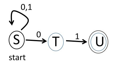
This is called a "Nondeterministic Finite Automaton", or NFA because in state S there are two options on input 0: we can stay in state S or transition to state T.
